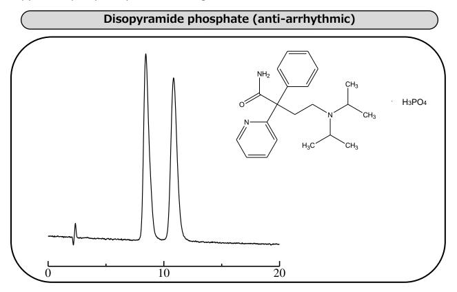
Column: ULTRON ES-OVM (5 µm) Column size: 150 mm L x 4.6 mm I.D.
