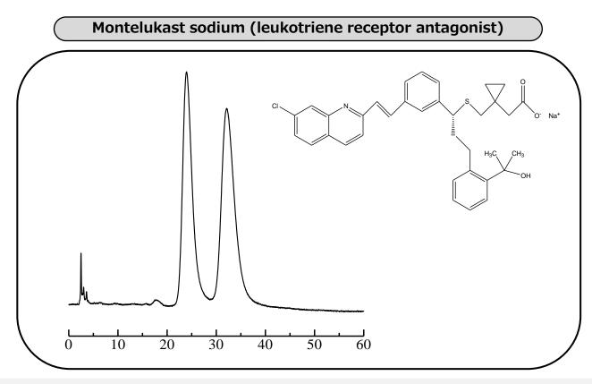
Column: ULTRON ES-OVM (5 µm) Column size: 150 mm L x 4.6 mm I.D. Mobile phase: 20 mM KH<sub>2</sub>PO<sub>4</sub> + H<sub>3</sub>PO<sub>4</sub> (pH 3.0)/CH<sub>3</sub>OH = 60/40 Flow rate: 1.0 mL/min
