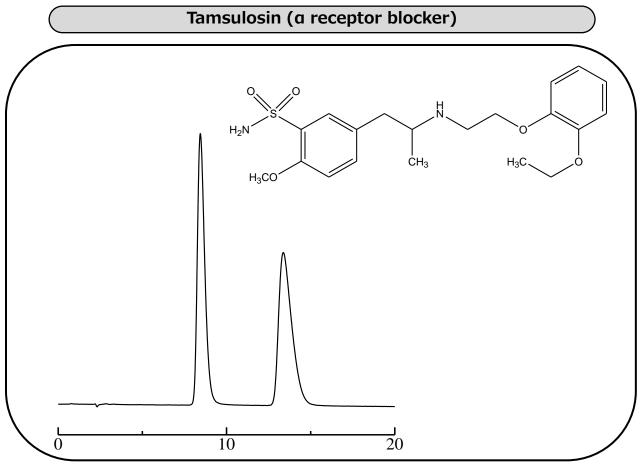
Column: ULTRON ES-OVM (5 µm) Column size: 150 mm L x 4.6 mm I.D.
