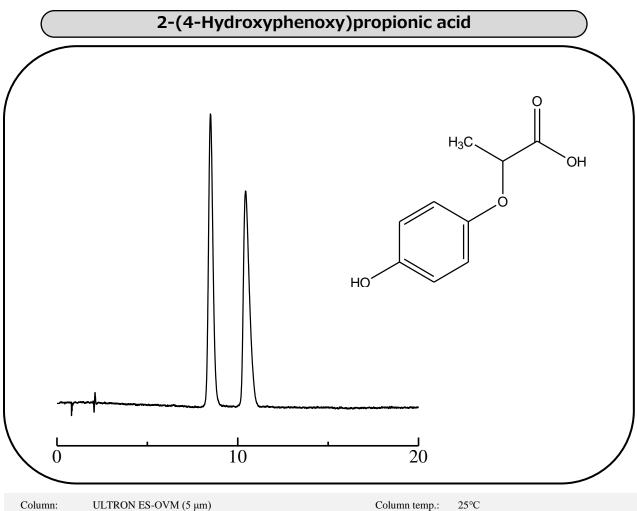
Column:ULTRON ES-OVM (5  $\mu$ m)Column size:150 mm L x 4.6 mm I.D.Mobile phase:20 mM KH<sub>2</sub>PO<sub>4</sub> + H<sub>3</sub>PO<sub>4</sub> (pH 3.0)/CH<sub>3</sub>CN = 90/10Flow rate:1.0 mL/min
