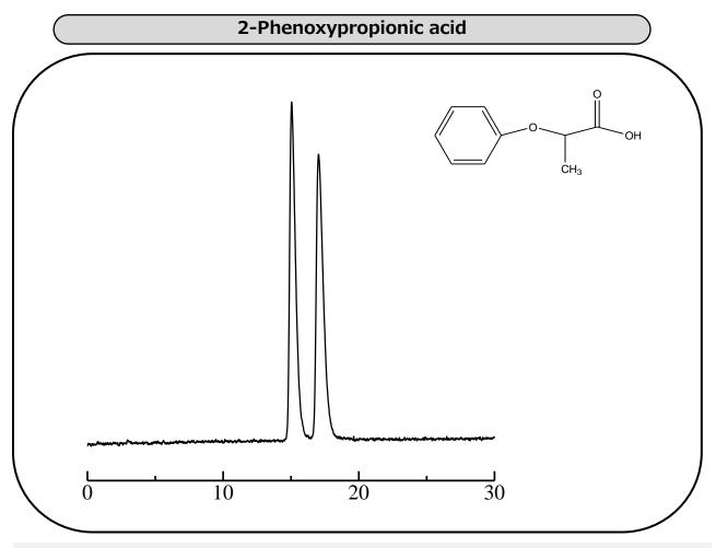
Column: ULTRON ES-OVM (5 μm) Column size: 150 mm L x 4.6 mm I.D.
