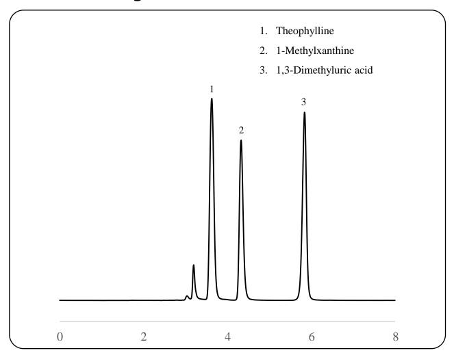
ULTRON AF-HILIC-CD (2 µm) Column temp.: 30°C Column: Flow rate: Column size: 150 mm L x 2.0 mm I.D. Mobile phase:  $10 \text{ mM CH}_3\text{CO}_2\text{NH}_4 \text{ (pH 6.8)/CH}_3\text{CN} = 13/87$ Injection vol.: 1.0 µL
