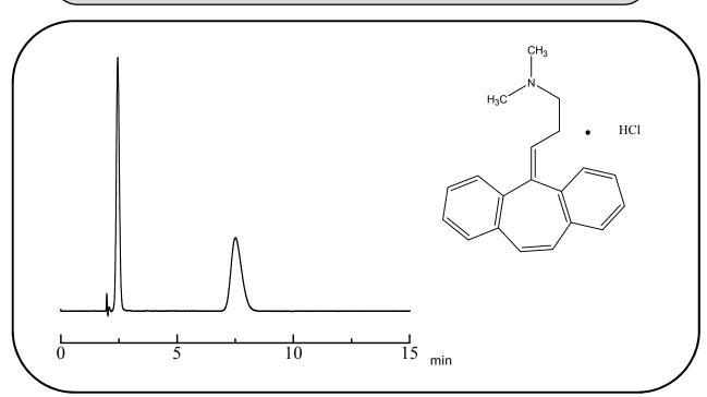
Column: ULTRON ES-OVM (5 μm) Column temp.: 25℃ Column size: 150 mm L x 4.6 mm I.D. Detection: UV-290 nm
