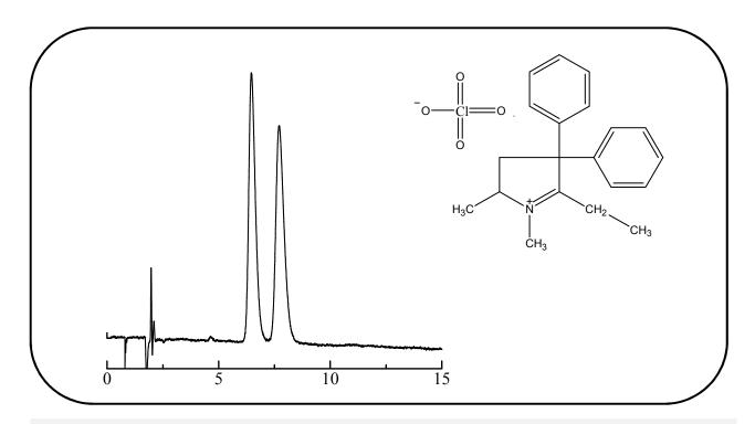
Column: ULTRON ES-OVM (5 µm) Column temp.:  $25^{\circ}\!\mathrm{C}$ Column size: 150 mm L x 4.6 mm I.D. Detection: UV-220 nm
