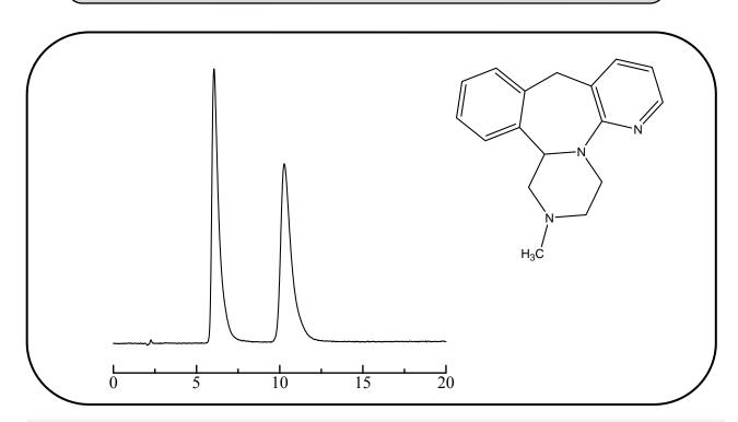
Column: ULTRON ES-OVM (5 µm) Column temp.:  $25^{\circ}\!\mathrm{C}$ UV-240 nm Column size: 150 mm L x 4.6 mm I.D. Detection:
