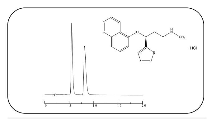
ULTRON ES-OVM (5 μm) Column temp.: 25℃ Column: Column size: 150 mm L x 4.6 mm I.D. Detection: UV-220 nm
