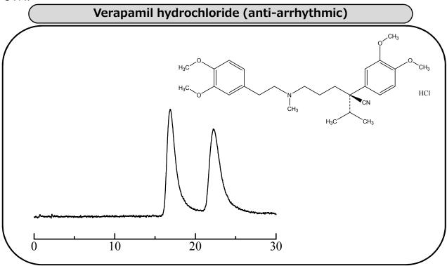
Column: ULTRON ES-OVM (5 μm) Column size: 150 mm L x 4.6 mm I.D.
