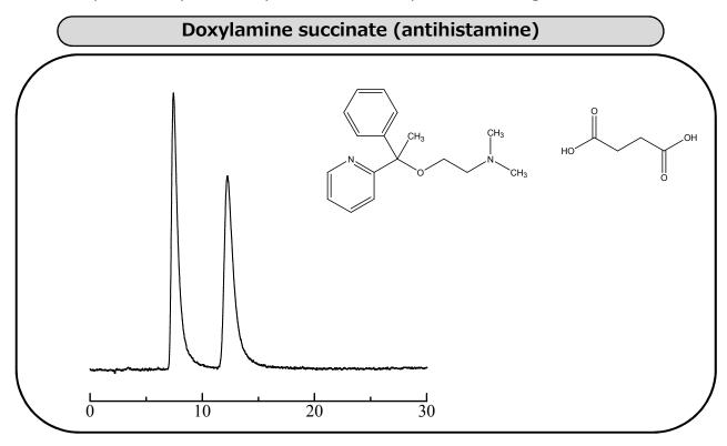
$\begin{array}{lll} \mbox{Column:} & \mbox{ULTRON ES-OVM (5 } \mbox{$\mu m$}) \\ \mbox{Column size:} & 150 \mbox{ mm L x } 4.6 \mbox{ mm I.D.} \\ \mbox{Mobile phase:} & 20 \mbox{ mM } \mbox{KH}_2\mbox{PO}_4 + 20 \mbox{ mM } \mbox{K}_2\mbox{HPO}_4 \mbox{ (pH } 6.0)/ \\ \end{array}$
