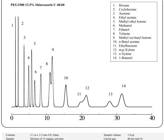
Column temp.: 70°C Injection port temp .: 200°C
