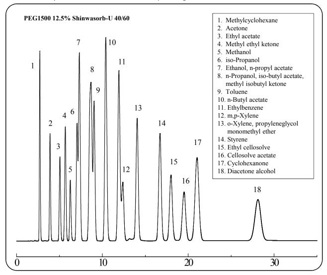
Column: 2.1 m x 3.2 mm I.D. Glass Mixture of 22 organic solvents Sample:
