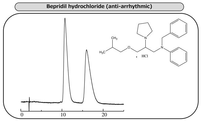
Column: ULTRON ES-OVM (5 µm) Column size: 150 mm L x 4.6 mm I.D.
