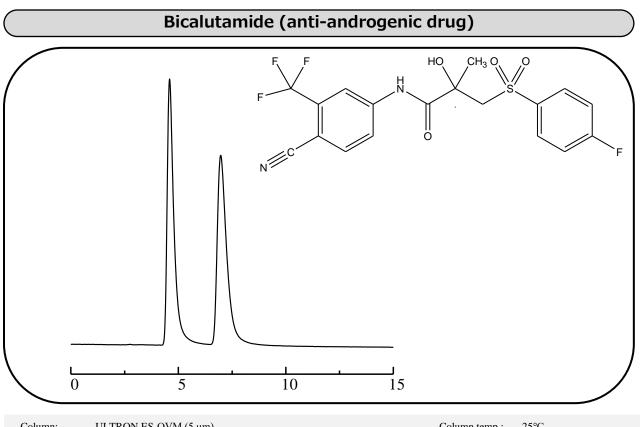
Column: ULTRON ES-OVM (5 µm) Column size: 150 mm L x 4.6 mm I.D. 20 mM KH<sub>2</sub>PO<sub>4</sub> + H<sub>3</sub>PO<sub>4</sub> (pH 3.0)/CH<sub>3</sub>CN = 87/13 Mobile phase: Flow rate: 1.0 mL/min
