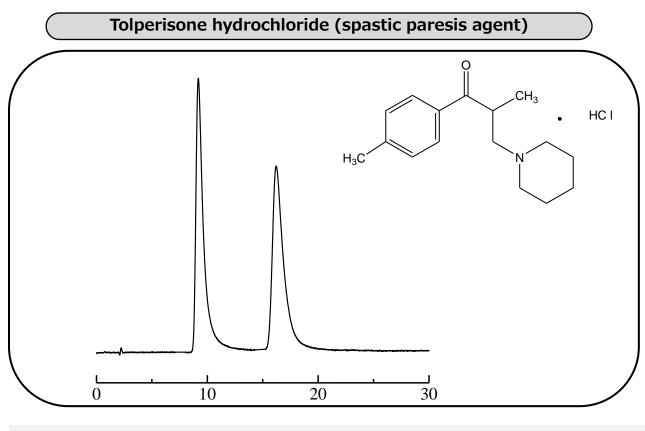
Column temp.: Detection: Sample: Injection vol.: 25°C UV-257 nm 200 mg/L (in ethanol) 2 μL
