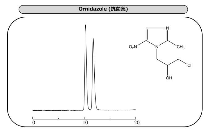
Column: ULTRON ES-OVM (5 μm) Column size: 150 mm L x 4.6 mm I.D.
