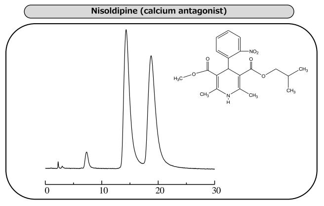
Mobile phase:  $20 \text{ mM KH}_2\text{PO}_4 + \text{H}_3\text{PO}_4 \text{ (pH } 3.0)/\text{CH}_3\text{CN} = 88/12$
