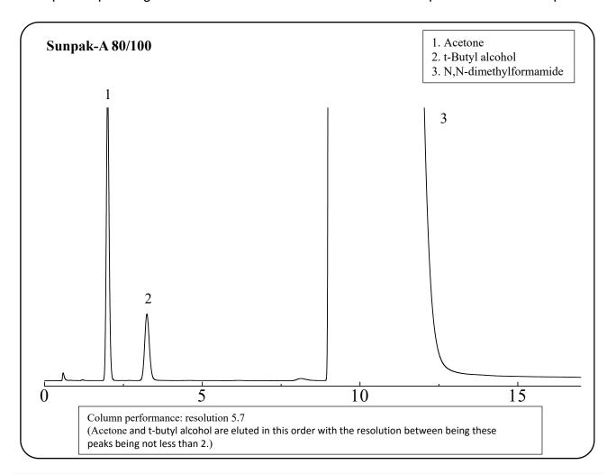
Column: 2.1 m x 2.0 mm I.D. Glass Sample volume: 1.0 μL Sample: Acetone, t-Butyl alcohol, N,N-Dimethylformamide Detector: FID 250
