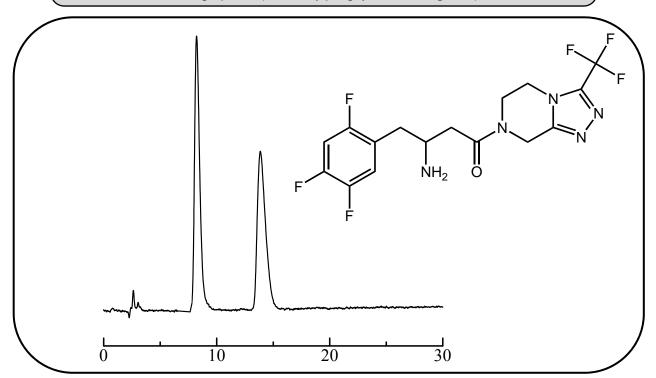
Column: ULTRON ES-OVM (5 µm) Column size: 150 mm L x 4.6 mm I.D.
