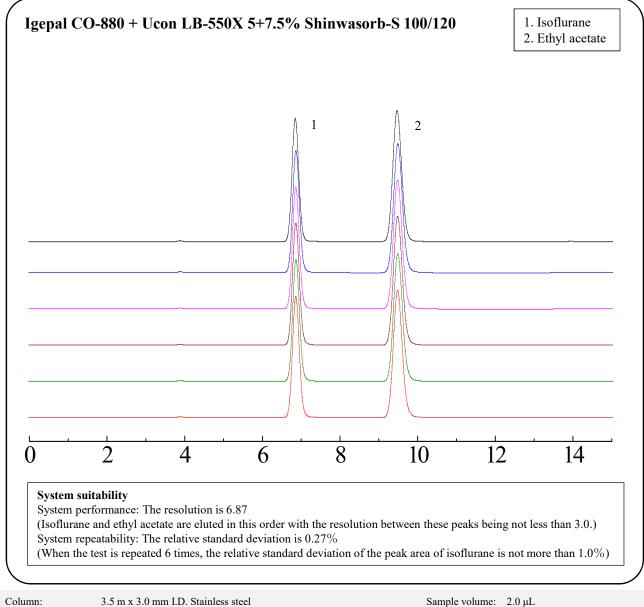
Column:3.5 m xSample:IsofluraColumn temp.:80°CInjection port temp.:200°CCarrier gas:37 mL
