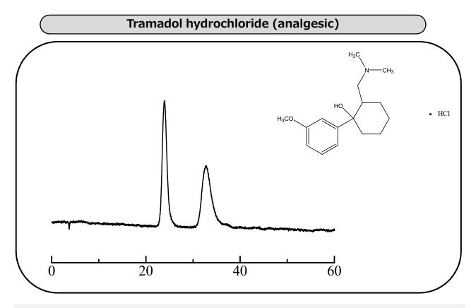
Column: ULTRON ES-PhCD-T (5 μm) Column temp.: 25°C Column size: 150 mm L x 6.0 mm I.D. UV-270 nm Detection:
