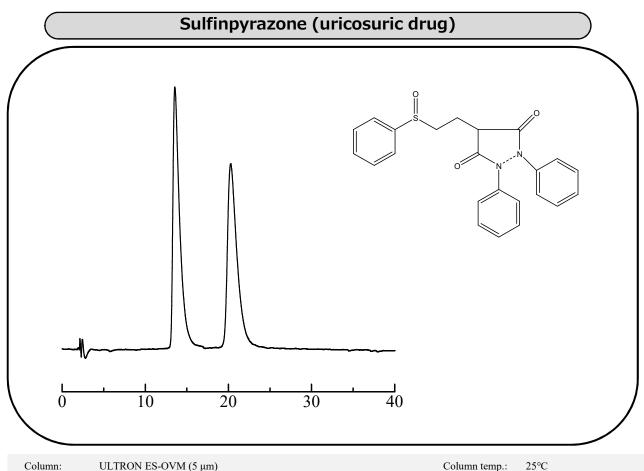
Column size: 150 mm L x 4.6 mm I.D. 10 mM CH<sub>3</sub>COONH<sub>4</sub> (pH 6.8)/CH<sub>3</sub>CH(OH)CH<sub>3</sub> = 95/5 Mobile phase: Flow rate: 1.0 mL/min
