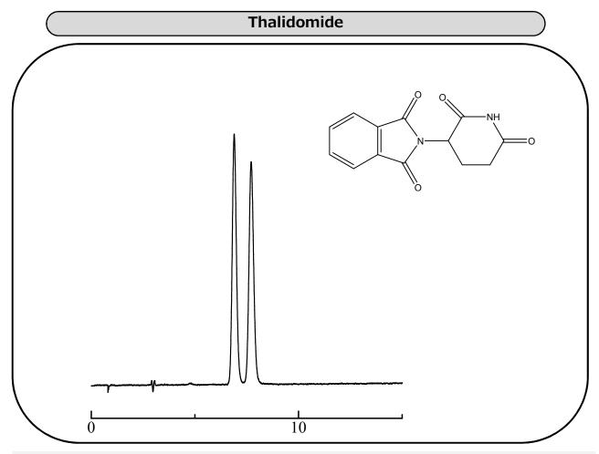
Column: ULTRON ES-OVM (5 µm) Column size: 150 mm L x 4.6 mm I.D.
