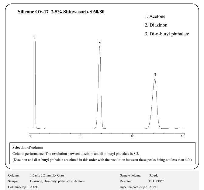
Carrier gas: 25 mL/min N2 (Adjust so that the retention time of diazinon is about 7 minutes.)
