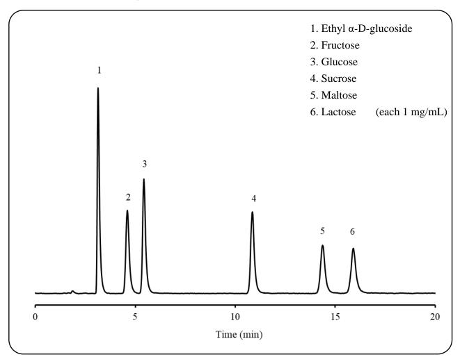
Column: ULTRON AF-HILIC-CD (2  $\mu$ m) Column temp.: 40°C Column size: 150 mm L x 2.0 mm I.D. Flow rate: 0.3 mL/min Mobile phase: 10 mM CH<sub>3</sub>CO<sub>2</sub>NH<sub>4</sub> (pH 6.8)/CH<sub>3</sub>CN = 12/88 Injection vol.: 1.0  $\mu$ L Detection: ELSD
