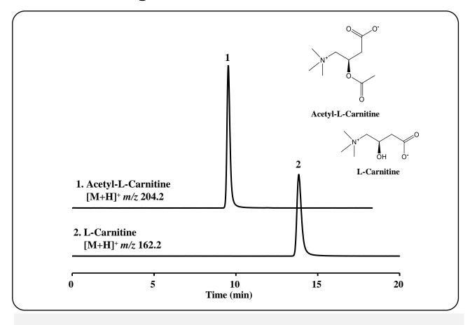
Column: ULTRON AF-HILIC-CD (2 μm)
