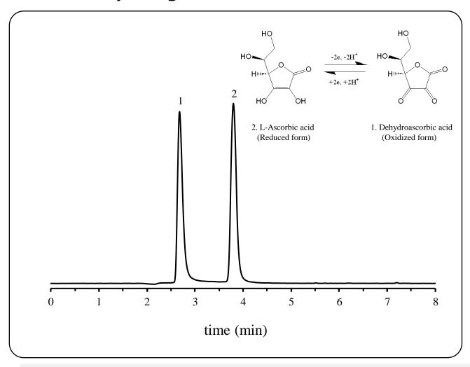
Column: ULTRON AF-HILIC-CD (2 μm)
