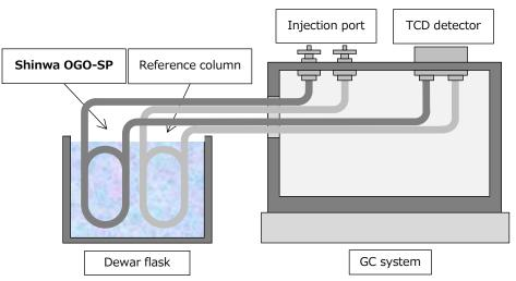
Note: In the case of a multi-filament TCD detector, in addition to the packed column for deuterium analysis, a reference column and connecting piping (e.g., GM-GF 2 x 1 mm I.D. 4 Nos) are required. For the reference column, we recommend "Shimalite Q". For a single-filament TCD detector, a reference column is not required.
