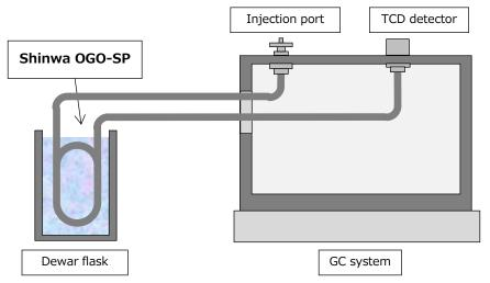
Note: In case of a single-filament TCD detector, in addition to the packed column for deuterium analysis, connecting piping (e.g., Reducing union 2 pcs, Ferrules and nuts 2 pcs each, Connecting piping 1000 mm x 0.5 mm I.D. x 2.0 mm O.D. 2 Nos) is required.
