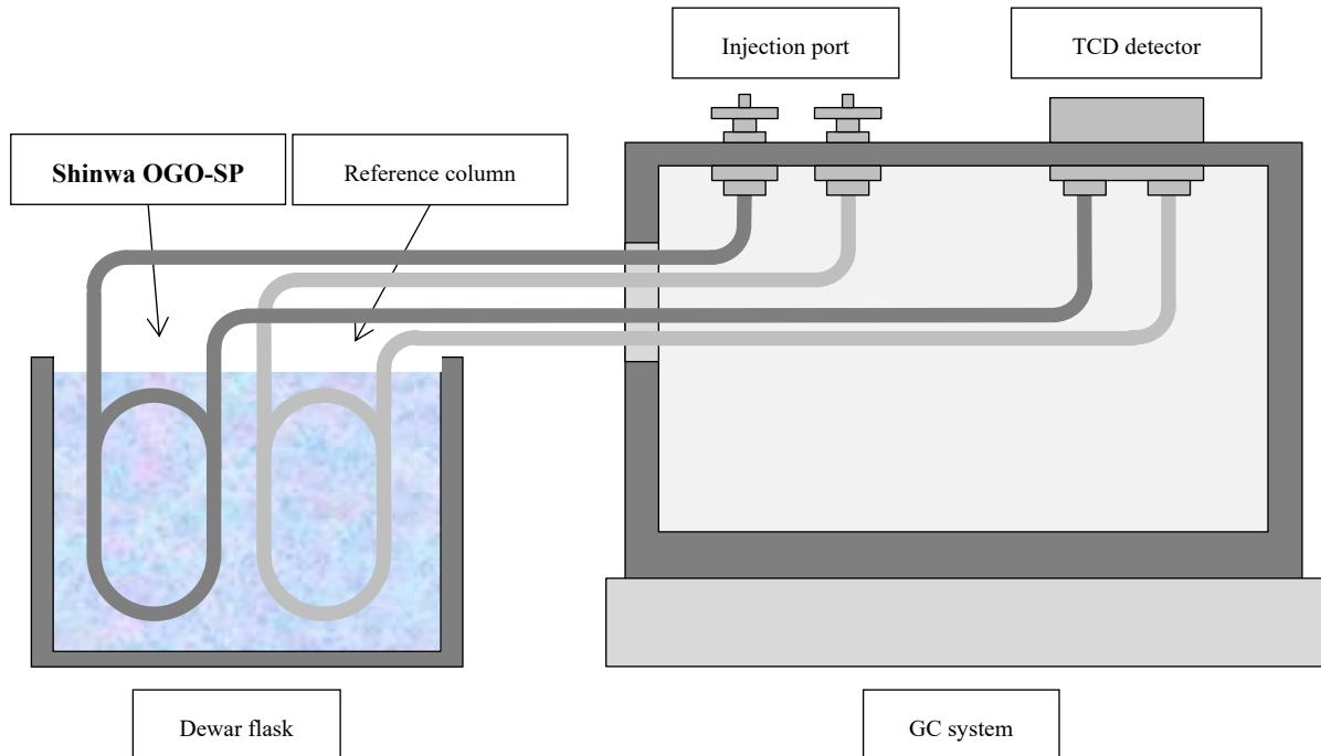
Note: In the case of a multi-filament TCD detector, in addition to the packed column for deuterium analysis, a reference column and connecting piping (e.g., GM-GF 2 x 1 mm I.D. 4 Nos) are required. For the reference column, we recommend "Shimalite Q". For a single-filament TCD detector, a reference column is not required.
