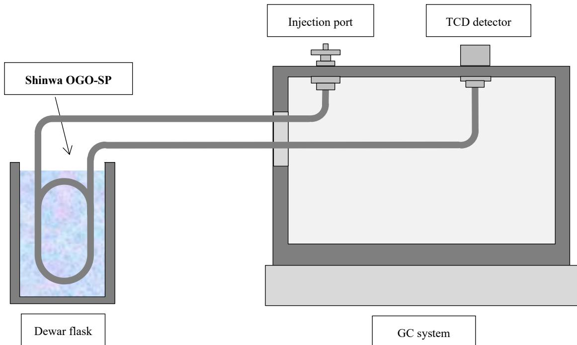
Note: In case of a single-filament TCD detector, in addition to the packed column for deuterium analysis, connecting piping (e.g., Reducing union 2 pcs, Ferrules and nuts 2 pcs each, Connecting piping 1000 mm x 0.5 mm I.D. x 2.0 mm O.D. 2 Nos) is required. If you have any questions, please contact our representative.
