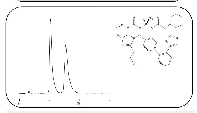
Column: ULTRON ES-OVM (5 µm) 150 mm L  $\times$  4.6 mm I.D. Column size:  $20 \text{ mM } \text{KH}_2\text{PO}_4/\text{CH}_3\text{CN} = 75/25$ Mobile phase:
