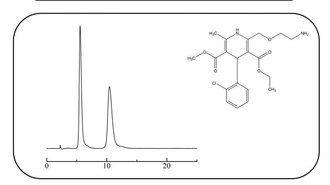
Column: ULTRON ES-OVM (5 µm) Column temp.: 25°C Column size: UV-237 nm 150 mm L x 4.6 mm I.D. Detection:
